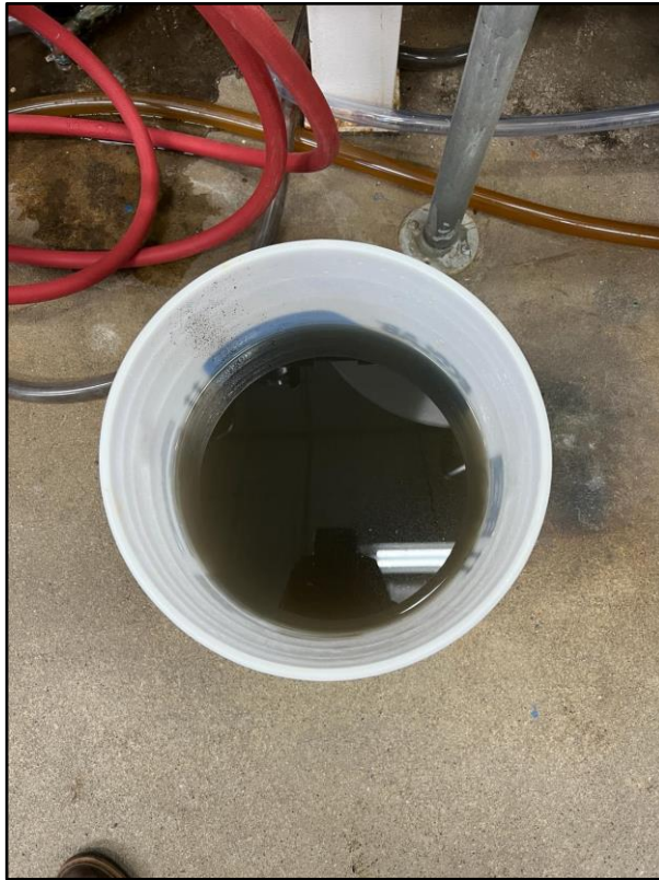
Figure 4: Filter 2 backwash water, February 6th.
