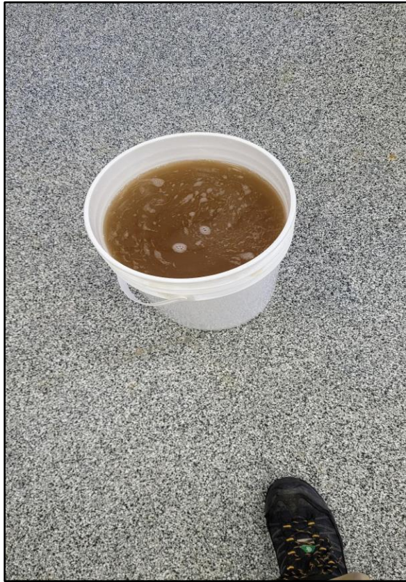
Figure 3: Filter 1 backwashed water, February 6th.
