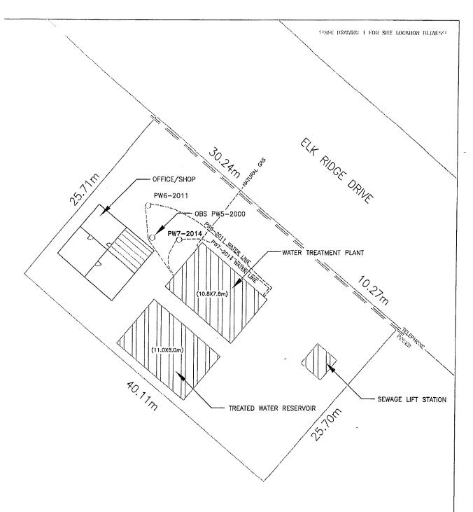
NOTES: PW7-2014 WATER LINE - 1.83 METRES OF 51mm HDPE PIPE CONNECTING PITLESS ADAPTER TO THE 38.1mm HDPE PIPE REUSED FROM PW5-2000.
